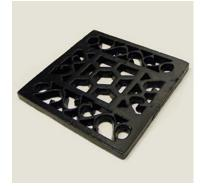
The photograph to the left shows a 125 x 125mm black cast-iron external vent. This event is to be used as the external visible grille detail for the mechanical extract for the cellar and is to be installed at low-level, just above ground on the north elevation.
