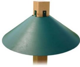
Galvanised steel cones fixed to drainpipes and telegraph poles would prevent cats from using them to climb over the buildings. It is recommended that the cones are 300mm in radius to be an effective cat barrier.
