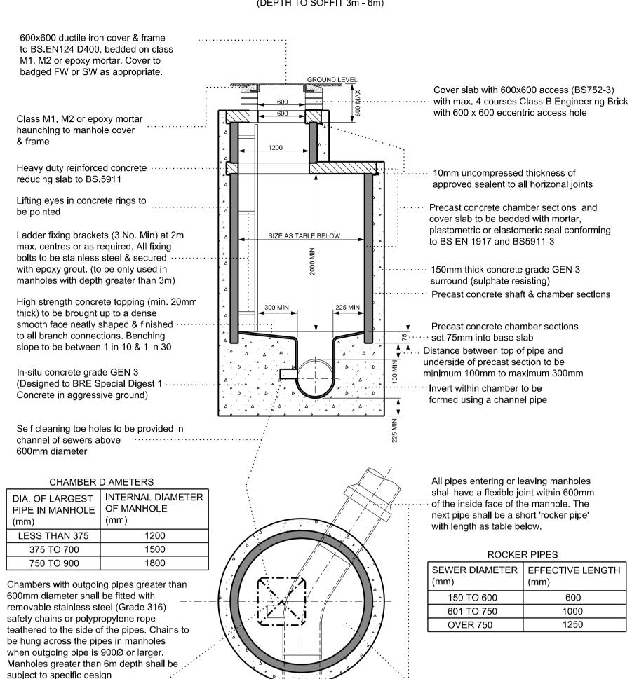
For manholes of 1800 dia of larger. Below 1800 dia chamber rings continue to cover slab (no shaft)
