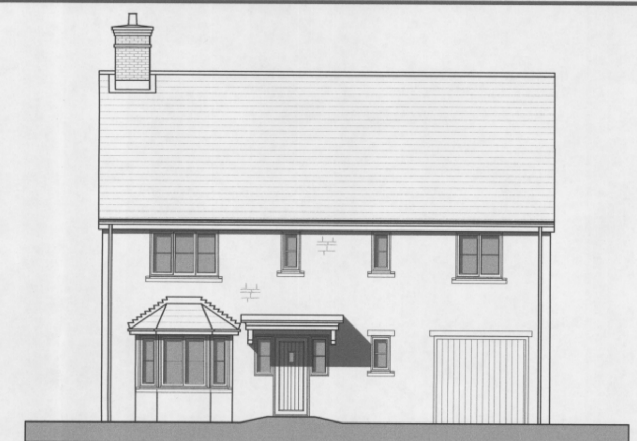
FRONT ELEVATION TYPE II - IRON STONE PLOT 71 & 73 READ AS. (PLOTS 70 & 72 READ HANDED)
