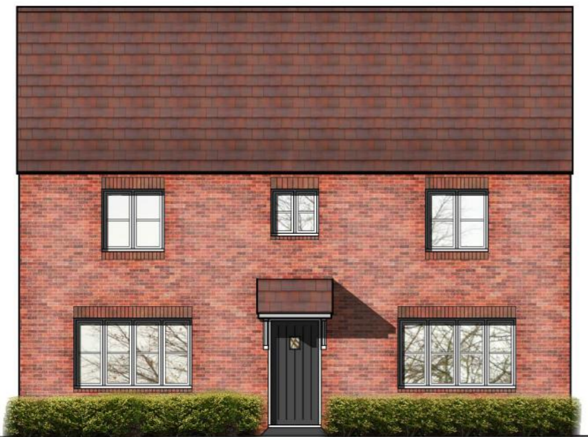
PW4008 Informal Brick Style Wall - Ibstock Brunswick Antique Roof - Sandcroft 20/20 roof tiles Flanders
