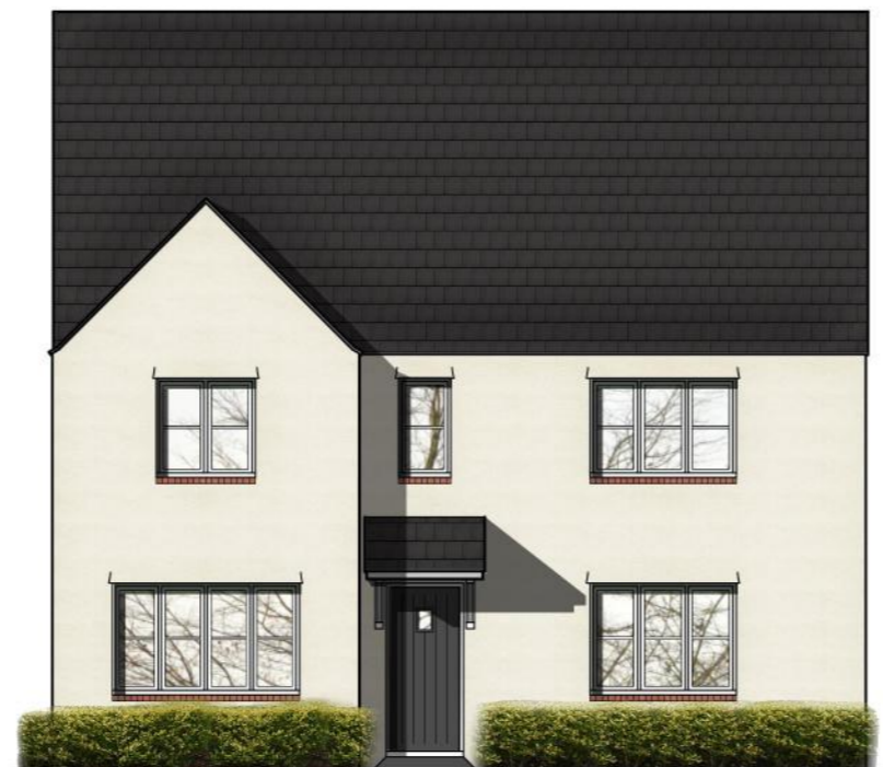
P501 Render Style Wall - SAS Europe Renders Sandy Earth Roof - Sandcroft 20/20 Grey
