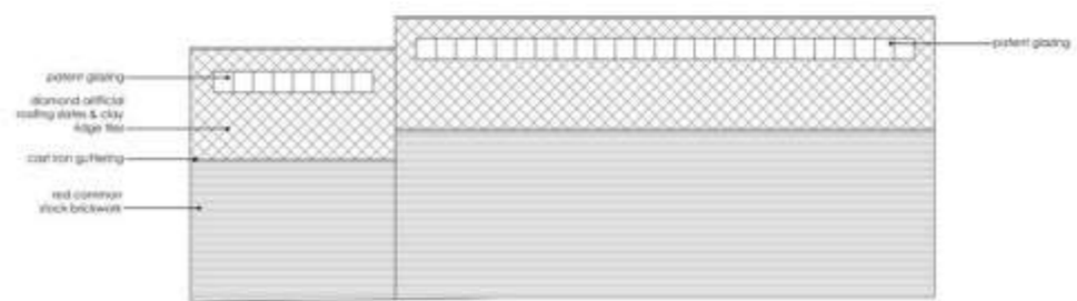
EXISTING NORTH ELEVATION
