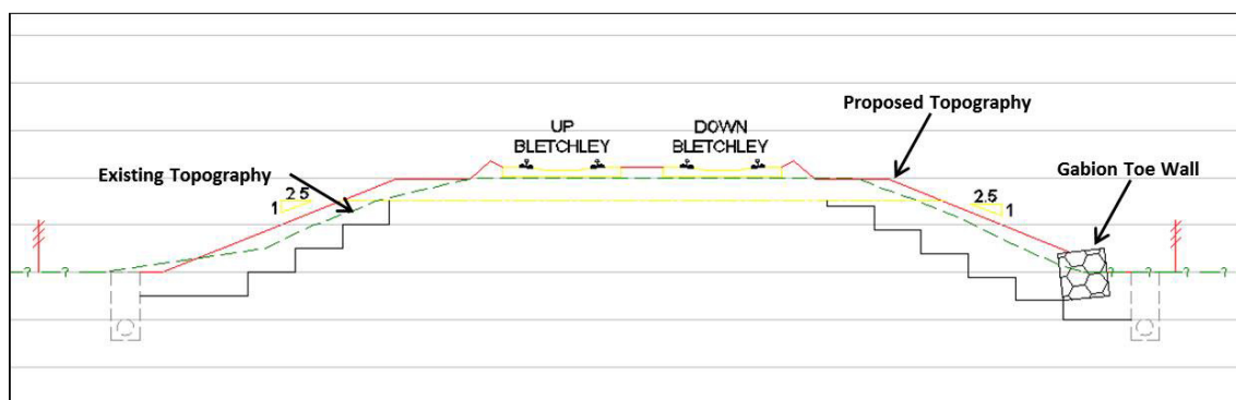
Figure 4 – Typical Cross Section Representing a Regrade Solution of the Left and Regrade and Gabion Toe Wall on the Right.
