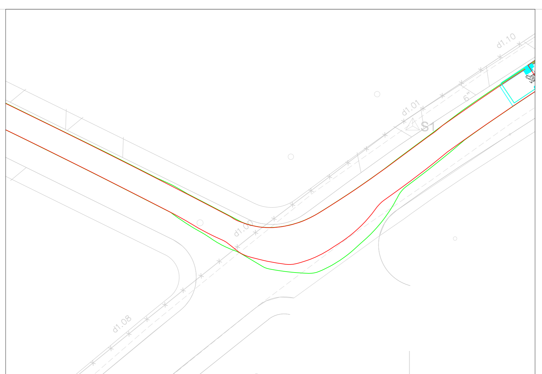
DETAIL C SHOWING 2.4m x 25m VISIBILITY SPLAY & RIGID BUS 25.0m FORWARD VISIBILITY SIGHTLINES SCALE 1:250
