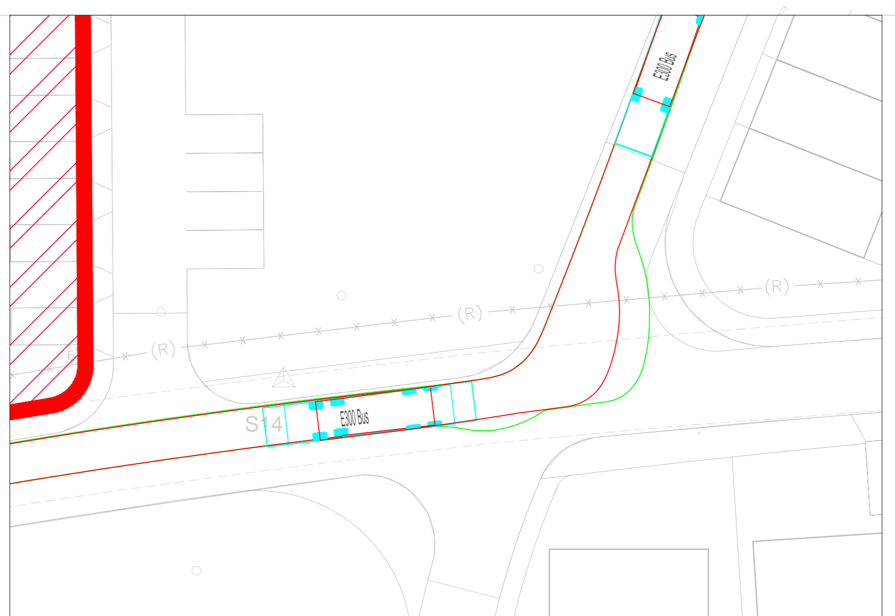
DETAIL D SHOWING 2.4m x 25m VISIBILITY SPLAY & RIGID BUS 25.0m FORWARD VISIBILITY SIGHTLINES SCALE 1:250
