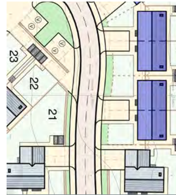
FIG. 149 | MINOR ACCESS ROAD
