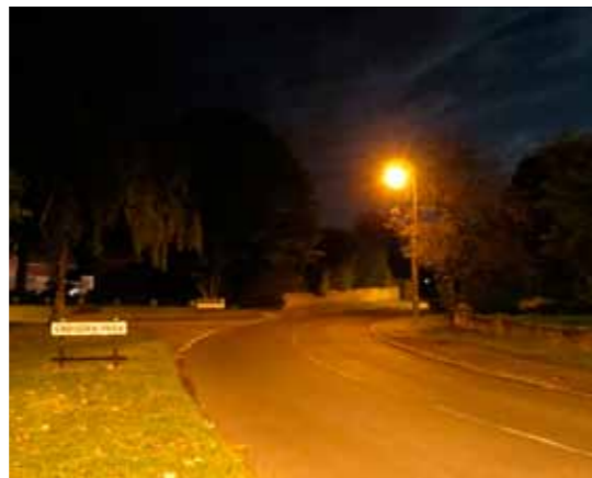
Cadogan Park - Night Pole-mounted High Pressure Sodium Light (at ~ 4.5m) Illuminance: 28 Lux
