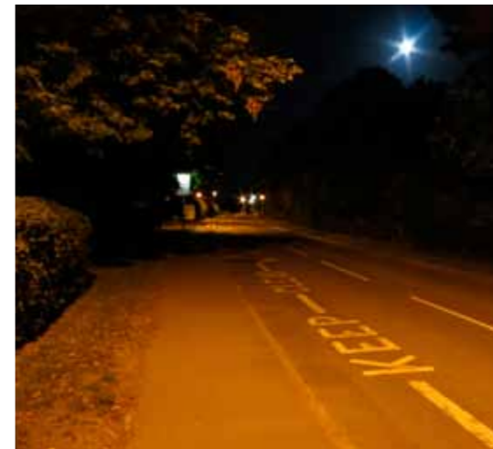
Shipton Rd (Marlborough School) - Night Pole-mounted High Pressure Sodium Light (at ~ 5m) Illuminance: 12 - 45 Lux Luminous Intensity of Light Source: 12000 cd
