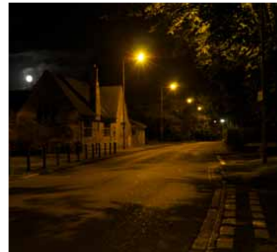
Woodstock Rd (A44) - Night High Pressure Sodium Street Light (at ~ 10m) Illuminance: 12 Lux Luminous Intensity of Light Source: 12000 cd
