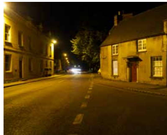
Woodstock St/ High St - Night Wall-mounted Flood Lights (at ~ 7m) Illuminance: 95 Lux Illuminance on neighbouring wall: 20 Lux (vertical)
