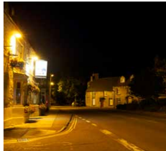
Woodstock St/ High St - Night Wall-mounted Flood Lights (at ~ 4.5m) Illuminance: 100 Lux Luminous Intensity of Pub sign: 40 cd
