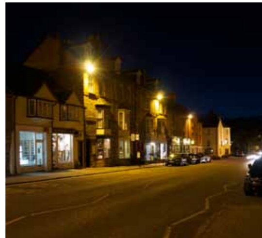
Woodstock St - Night Wall-mounted Flood Lights (at ~ 9m) Illuminance: 65 Lux Excessive lighting on pavement
