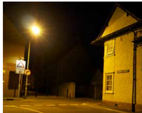
Union St/ Hensington Rd - Night High Pressure Sodium Street Light (at ~ 7m) Illuminance: 70 Lux Luminous Intensity of Light Source: 1200 cd
