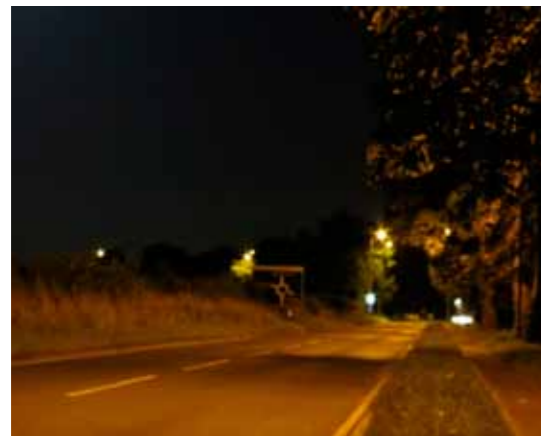
Woodstock Rd (A44) - Night High Pressure Sodium Street Light (at ~ 10m) Illuminance: 20 Lux
