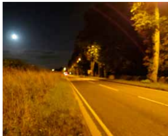
Woodstock Rd (A44)/ Churchill Gate - Night High Pressure Sodium Street Light (at ~ 10m) Illuminance: 20 Lux Luminous Intensity of Light Source: 750 cd
