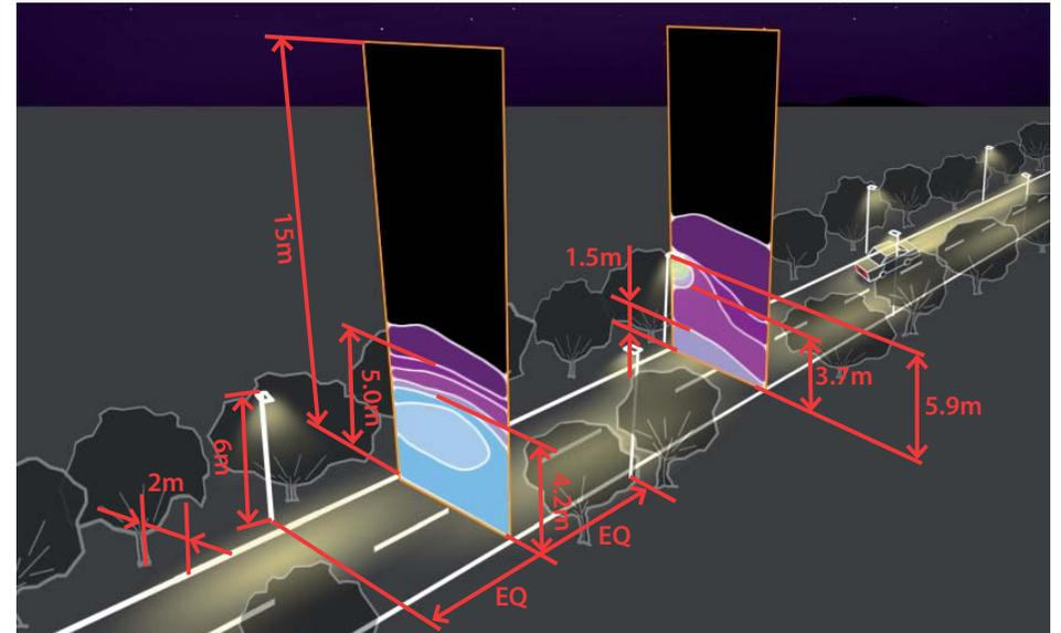
Illustration showing vertical calculation surface inserted into DIALUX computer model.
