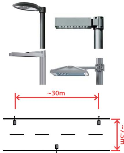
Suitable luminaire types and recommended mounting arrangement.
