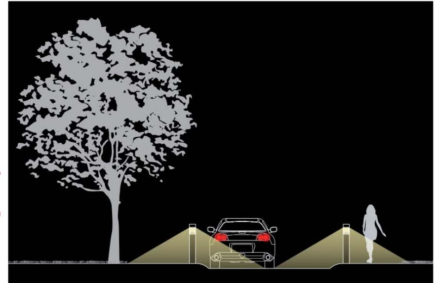
Sketch cross-section of tertiary road showing indicative light distribution from luminaires.
