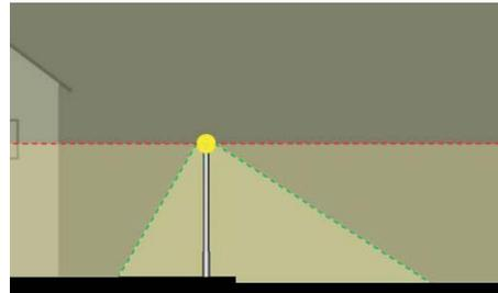
Luminaires that emit light above the horizontal plane should not be used.
