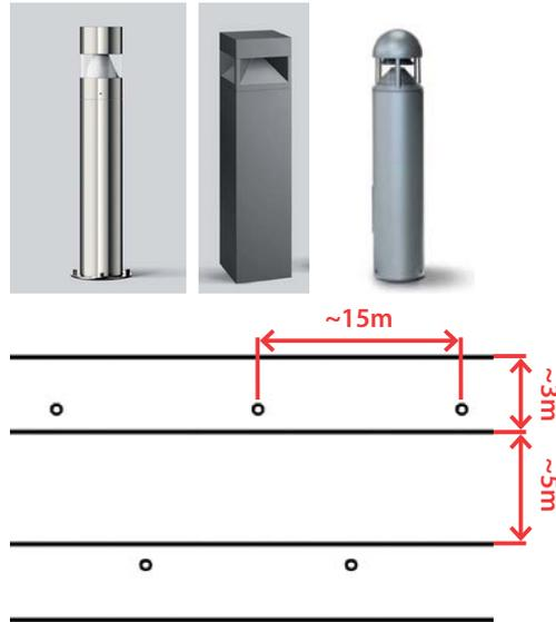
Suitable luminaire types and recommended mounting arrangement.
