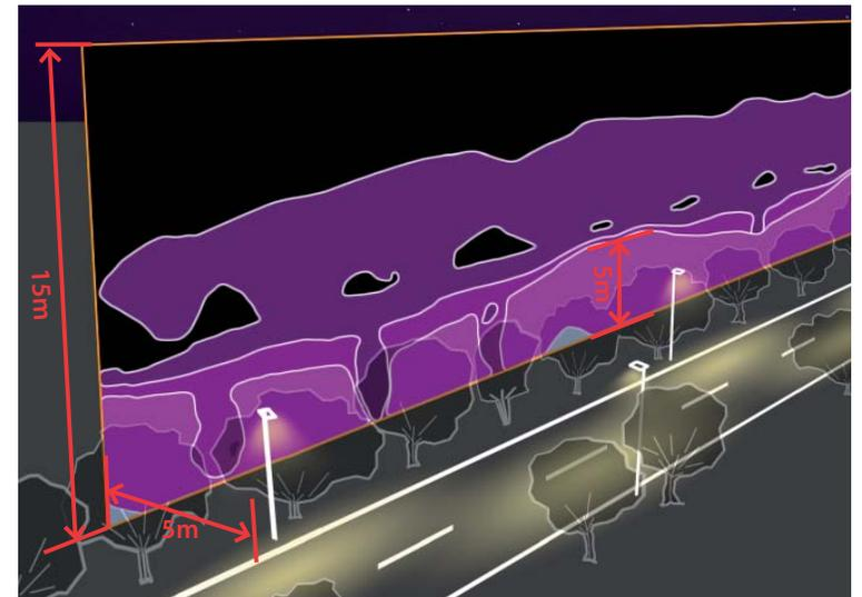
Illustration showing vertical calculation surface inserted into DIALUX computer model.
