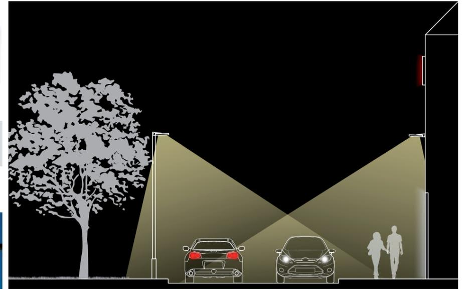
Sketch section showing wall mounted luminaires on retail units in combination with column mounted units
