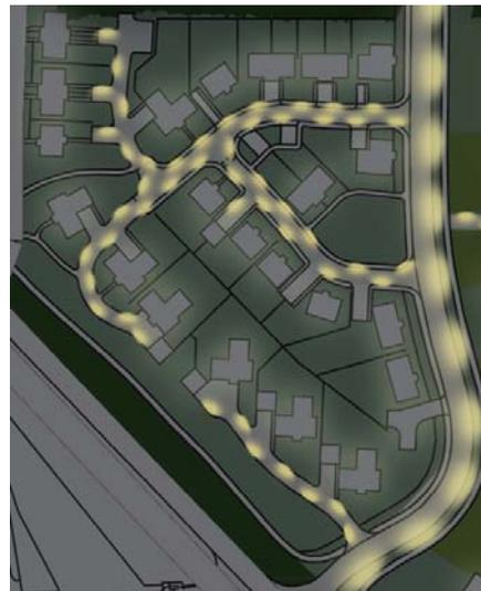
Sketch plan showing lighting arrangement for secondary and tertiary roads
