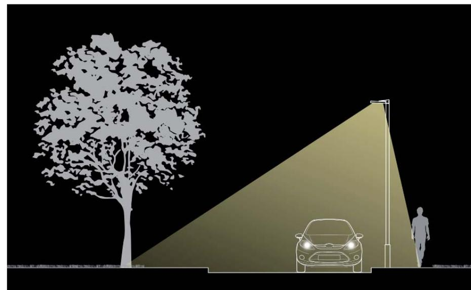
Sketch cross-section of secondary road showing indicative light distribution from luminaires.
