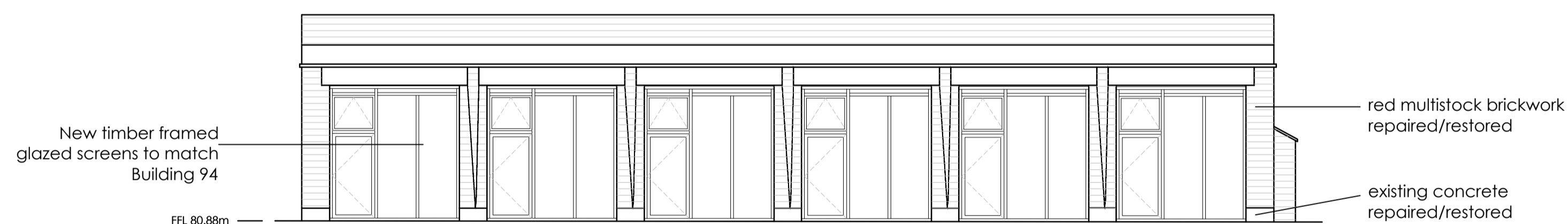
BUILDING 112 West Elevation - Proposed
