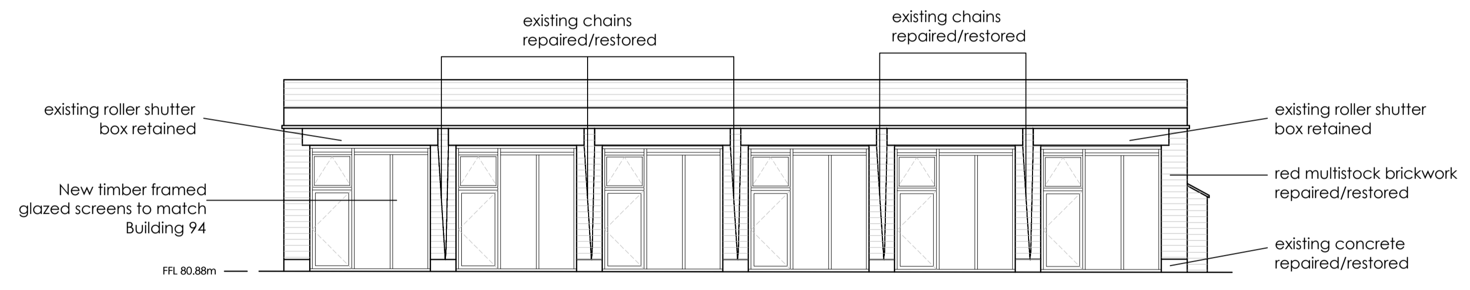
BUILDING 112 West Elevation - Proposed
