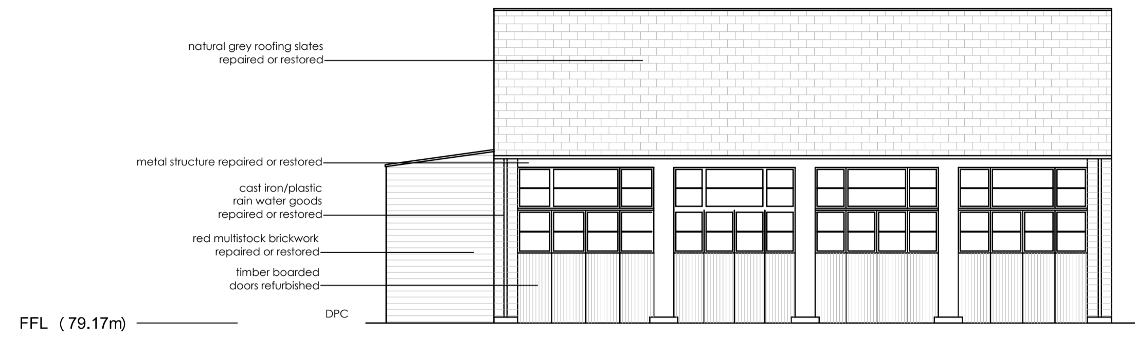
BUILDING 135 South West Elevation- Proposed
