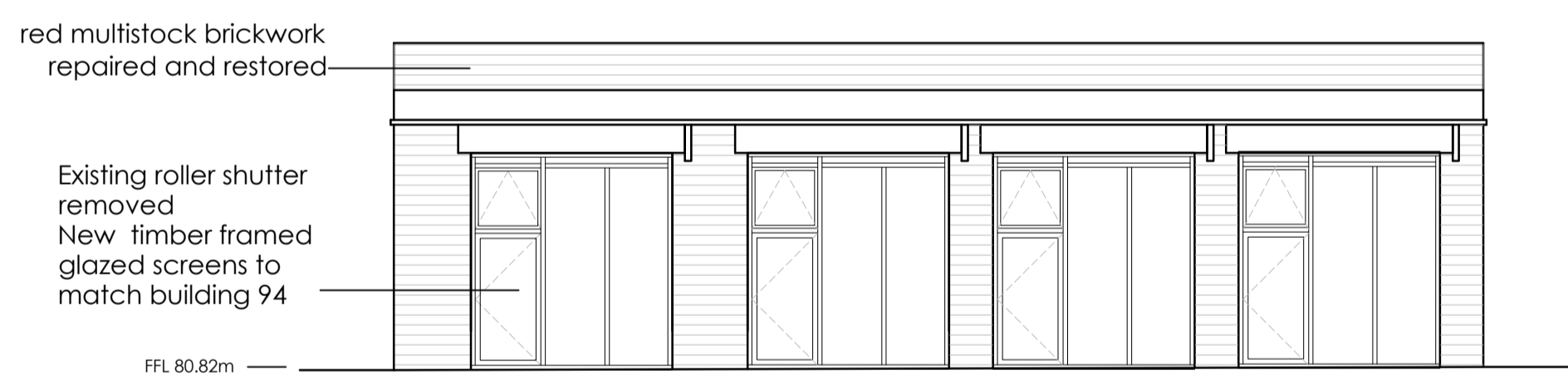
BUILDING 118 West Elevation-Proposed
