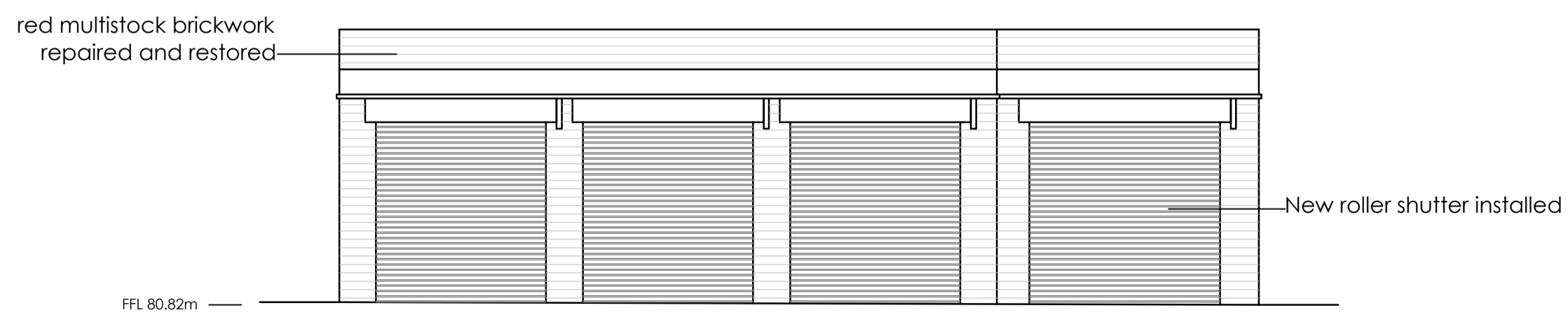
BUILDING 118 East Elevation-Proposed
