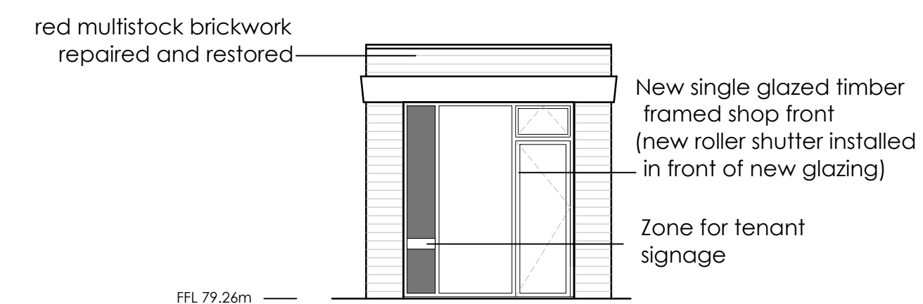
BUILDING 133 West Elevation-Proposed
