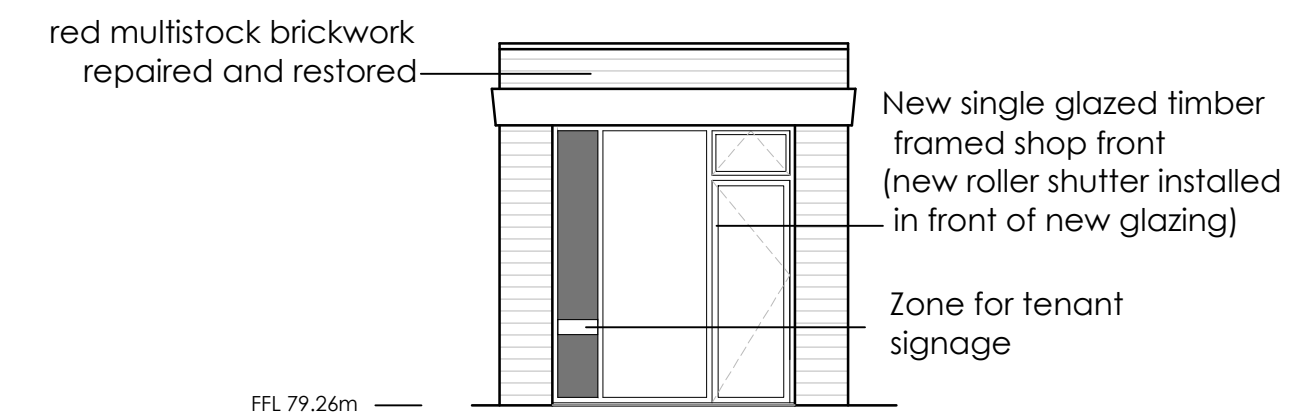
BUILDING 133 East Elevation-Proposed
