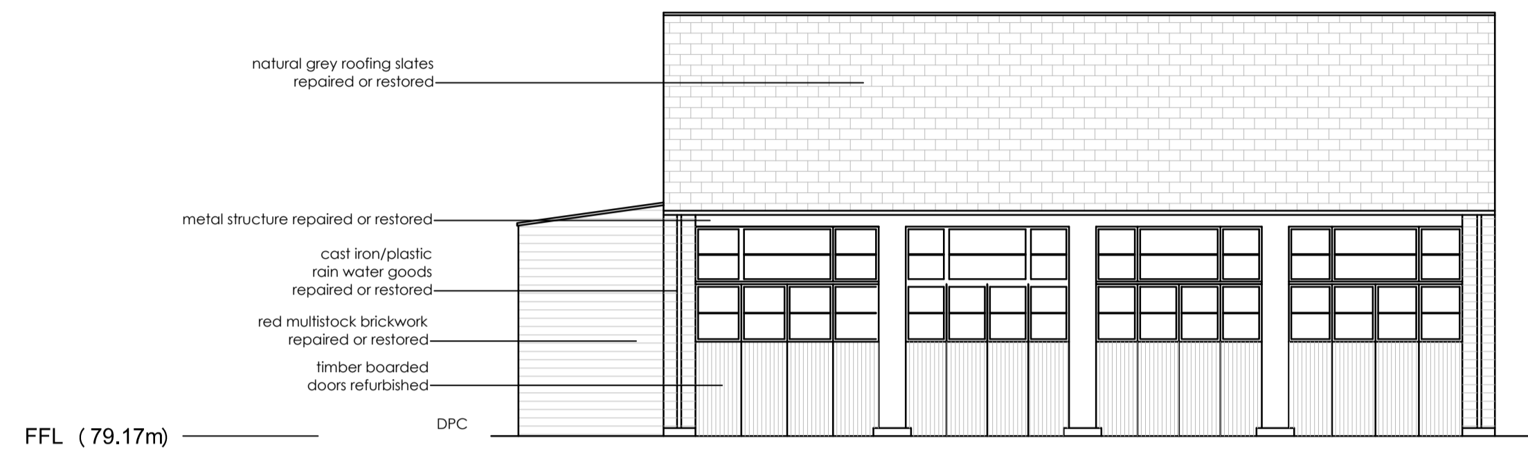
BUILDING 135 South West Elevation- Proposed
