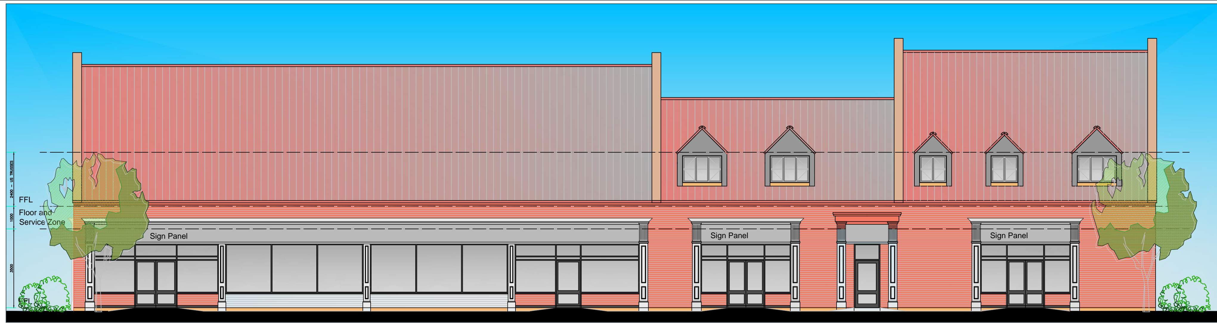
Shopfront Elevation Retail Unit A - single storey Retail Unit B with 2 Bed Apartment over Access to Apartments Surgery with 2 no. 2 Bed Apartments over
