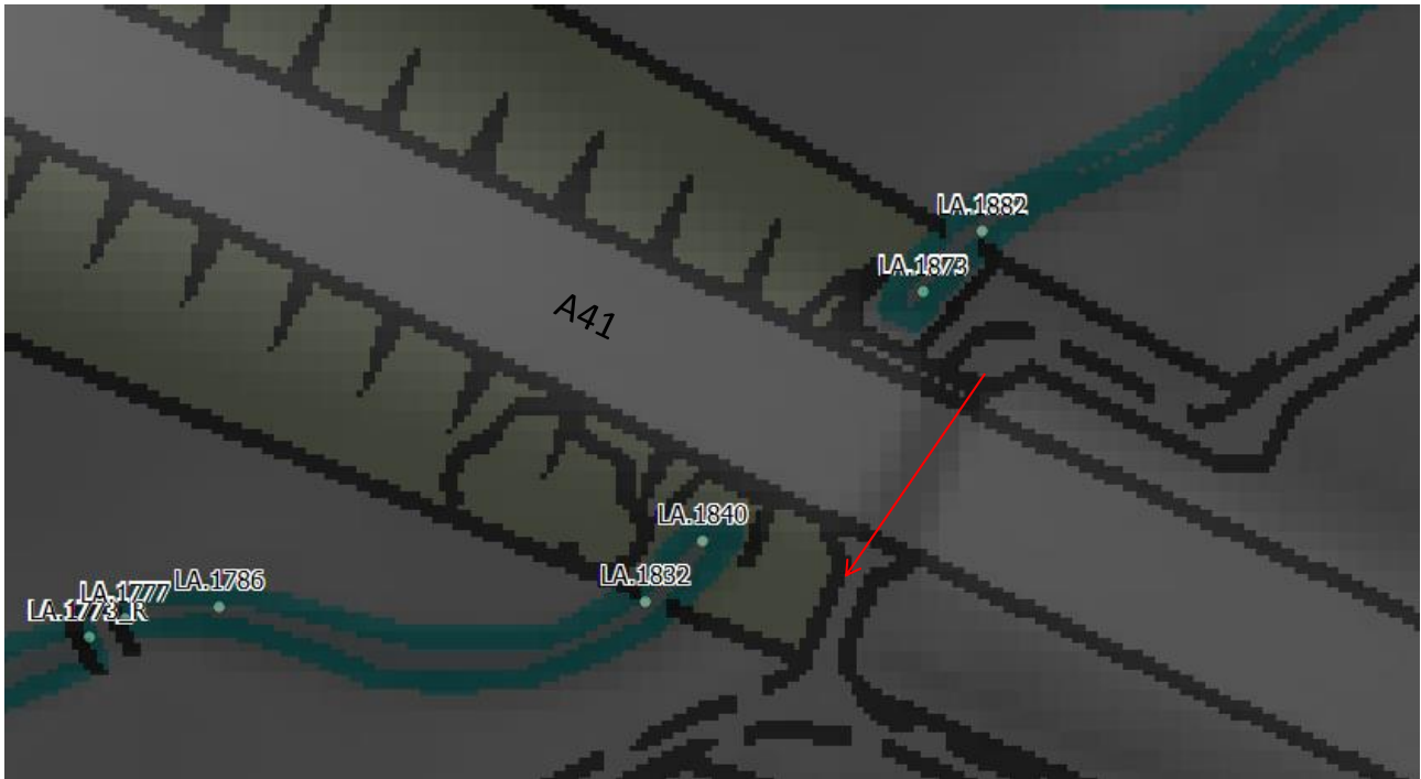
Figure 13 – 2D Flow Route not Originally Modelled within the PBA Model shown as Red Arrow (This has been modelled within this updated model simulation, HX link lines were changed to allow consideration of this flow route).
