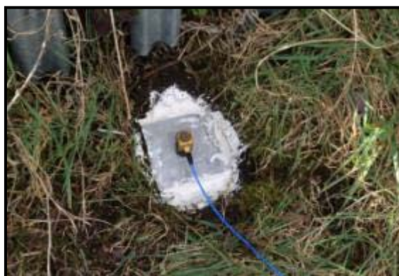
Figure 6. Example Measurement Position Accelerometer Set Up
