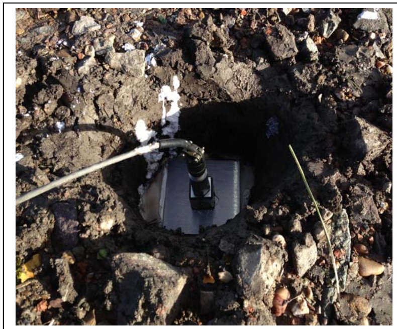
Figure 8. Example Measurement Position Accelerometer Set Up
