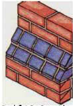
Example Illustration - Corner corbel detail
