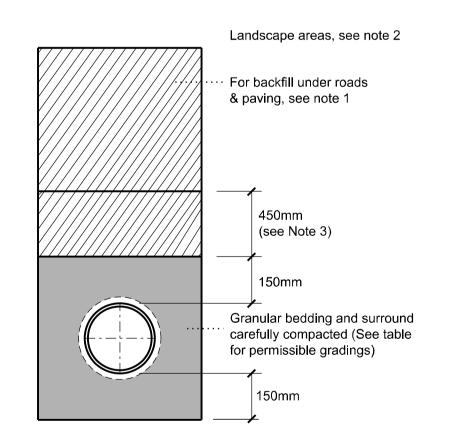
**CLASS S BEDDING DETAIL** (Rigid Pipes)
