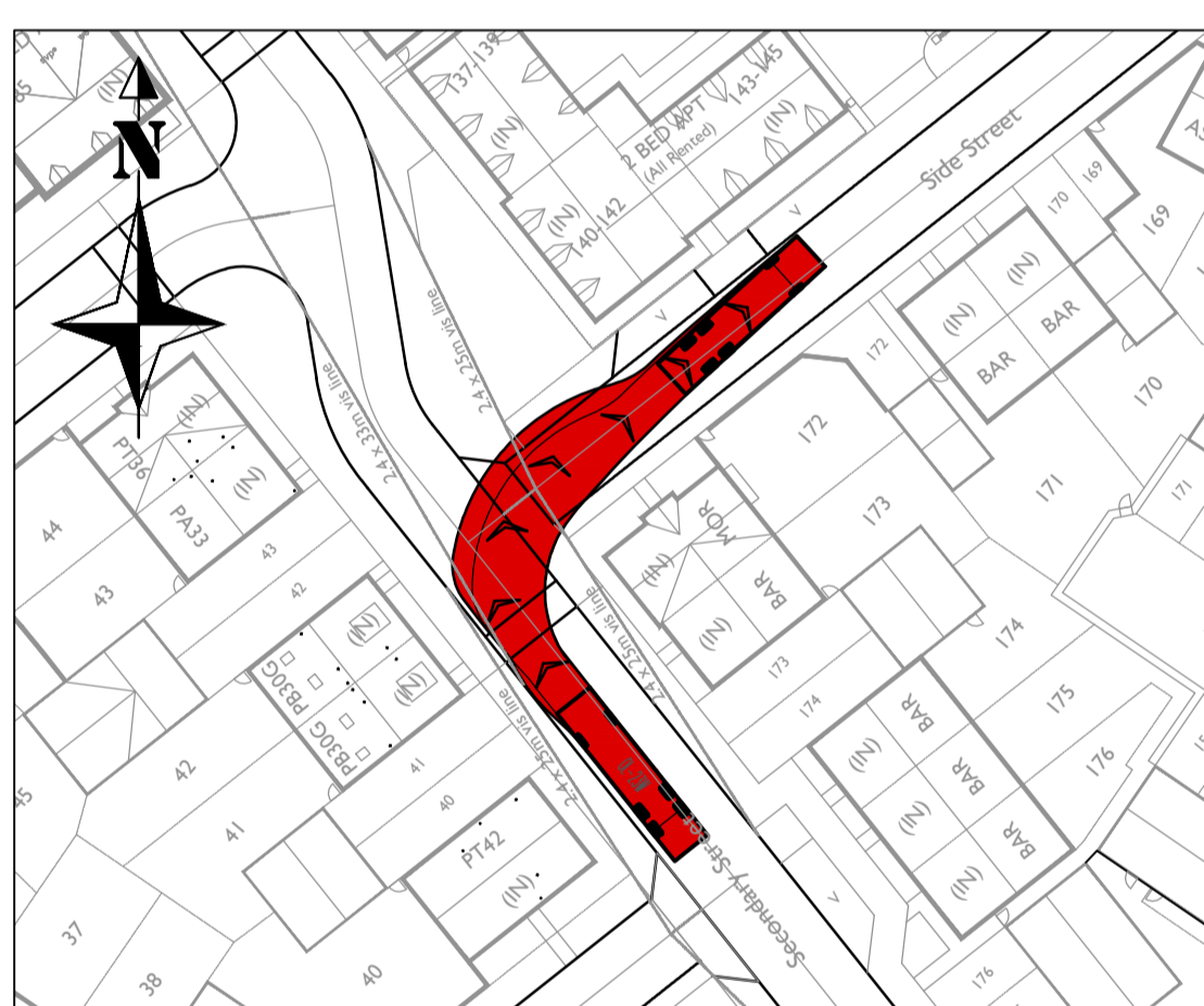
Refuse Vehicle Turning Right into junction of Roads 2 & 9
