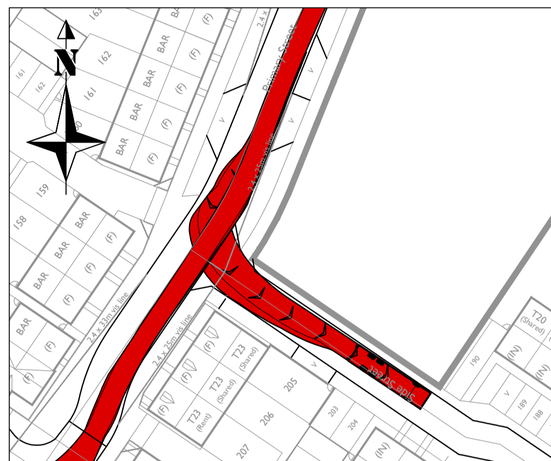
Refuse Vehicle Turning Left into junction of Roads 1 & 2 (East)
