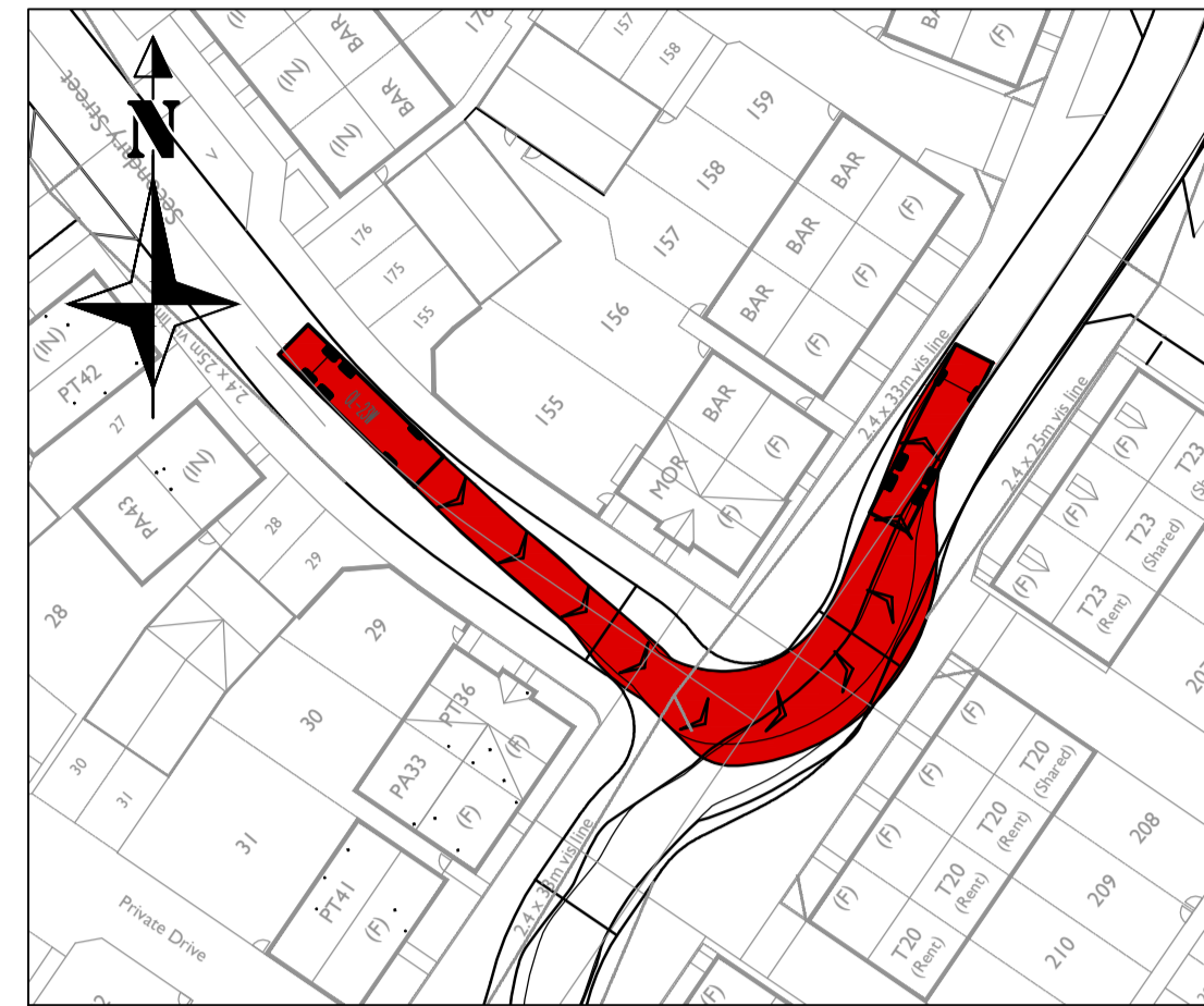
Refuse Vehicle Turning Left into junction of Roads 2 & 1
