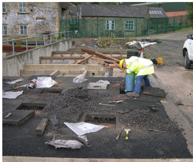
Figure 3 - In situ density tests post-trafficking.
