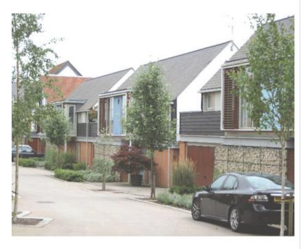
**LEFT** A shared surface street in Waterside, Chesterfield conveys the friendly 'mews-like' setting desired for all Urban Lanes at Graven Hill. Narrow plot frontages & the removal of designated highway zones (e.g. footways) are key design principles to achieving this.
