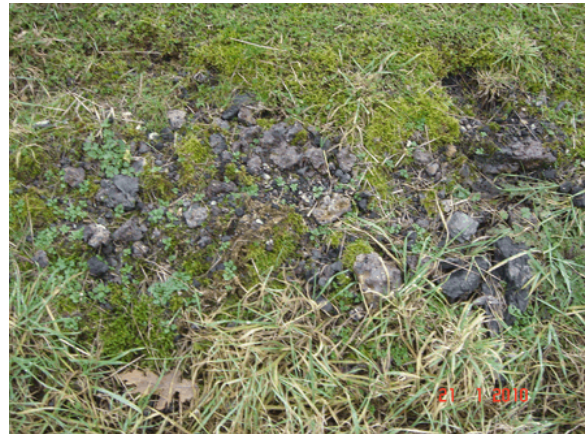
Plate 20: Clinker and Slag Material noted in the Railway Line Embankment
