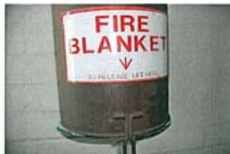
Photo 8 – 1.08 Lobby – Strongly Presumed asbestos blanket (fire)
