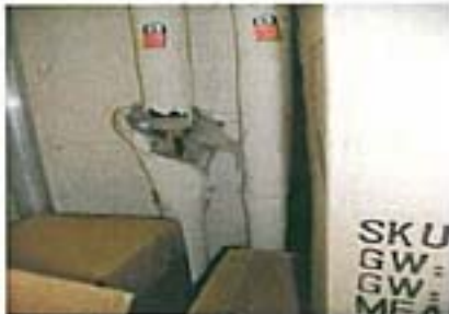
Photo 1 – 1.24 Store Room – Sample 1: Paper lining to pipework – Chrysotile
