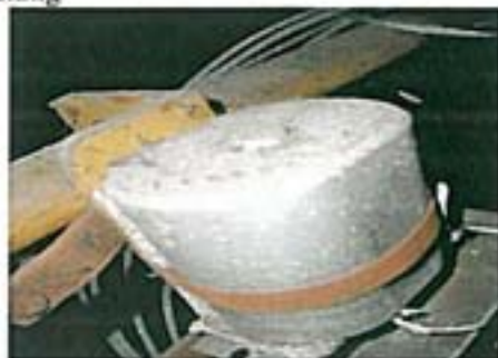
Photo 23 – 2.01 Roof Void – Sample 11: Rope (in switch box x4) also used as backing packing
