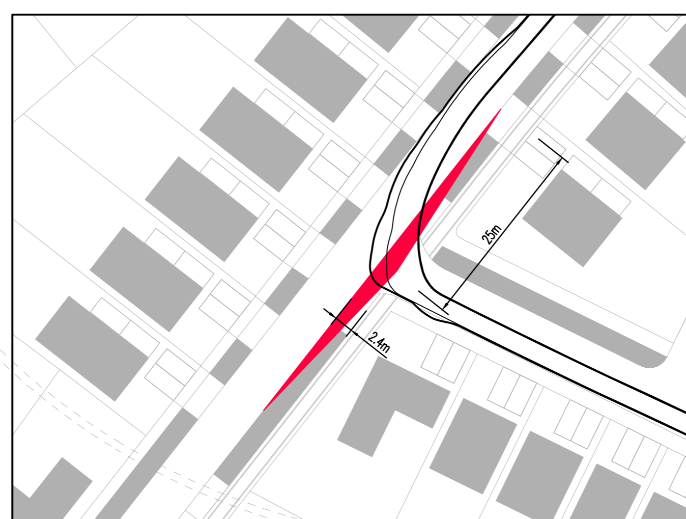
DETAIL D SHOWING 2.4m x 90m VISIBILITY SPLAY SCALE 1:500
