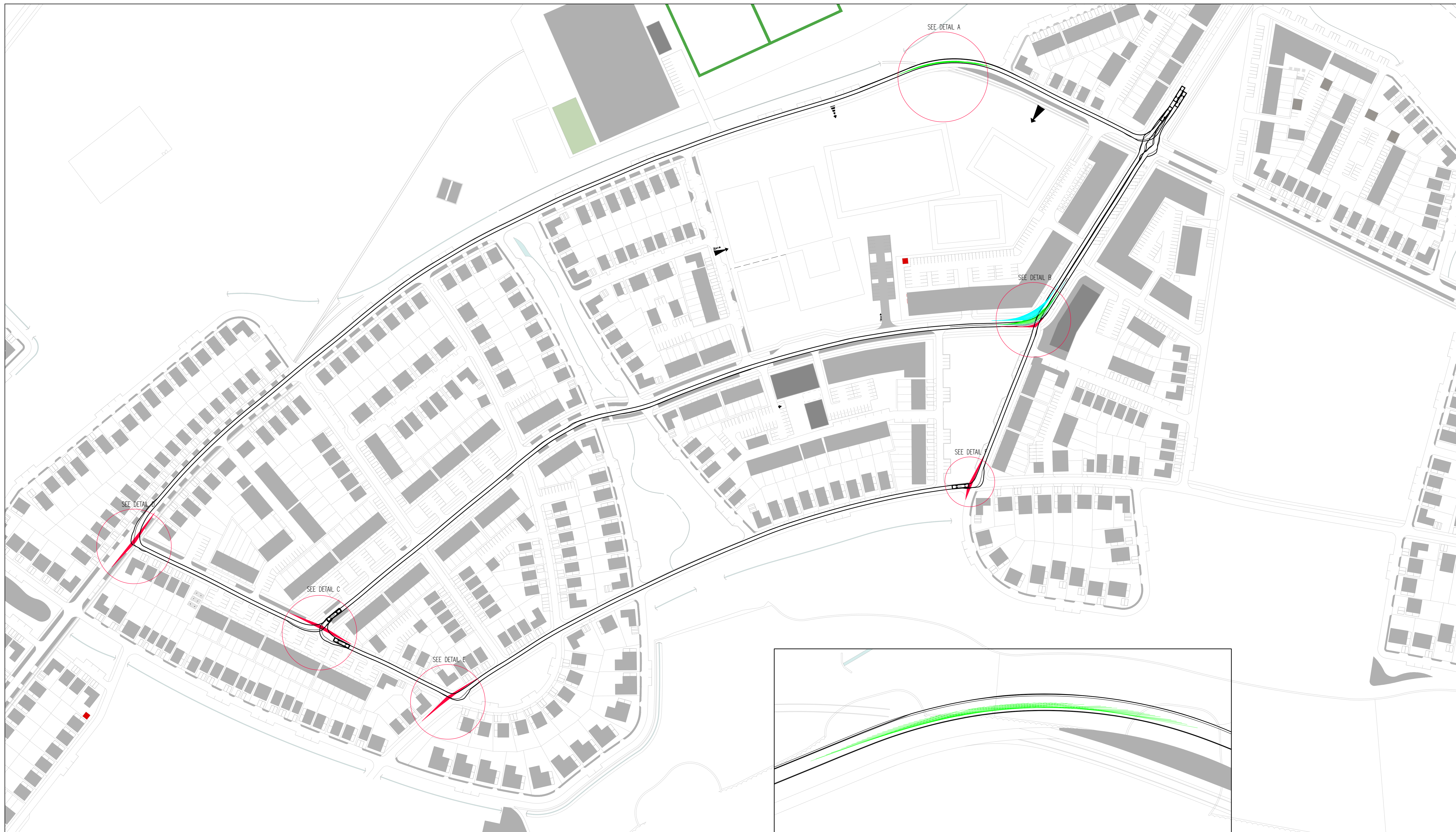
DETAIL A SHOWING RIGID BUS 25.0m FORWARD VISIBILITY SIGHTLINES SCALE 1:500
