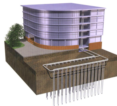
Figure 4.6: Ground Source Heat Pump System
