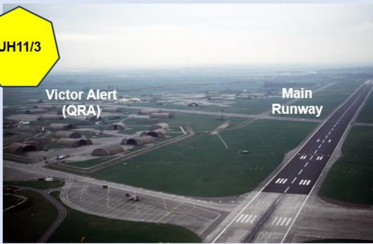
RAF Upper Heyford. Between 1950 and 1953 the main runway was widened and extended from 3500 feet (1067m) to 9604 feet (2927m). The closeness of villages to the runway caused noise and the danger of crashes during take-offs and landings.
