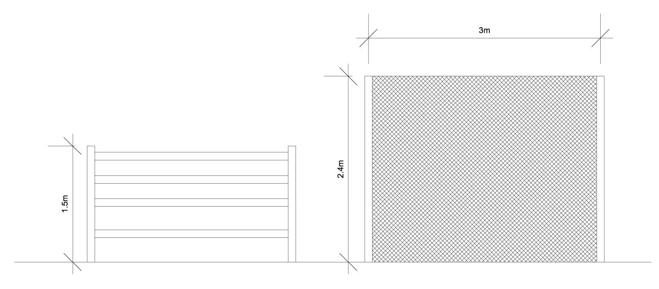
Timber & Post Rails Chain-link on Concrete Posts
