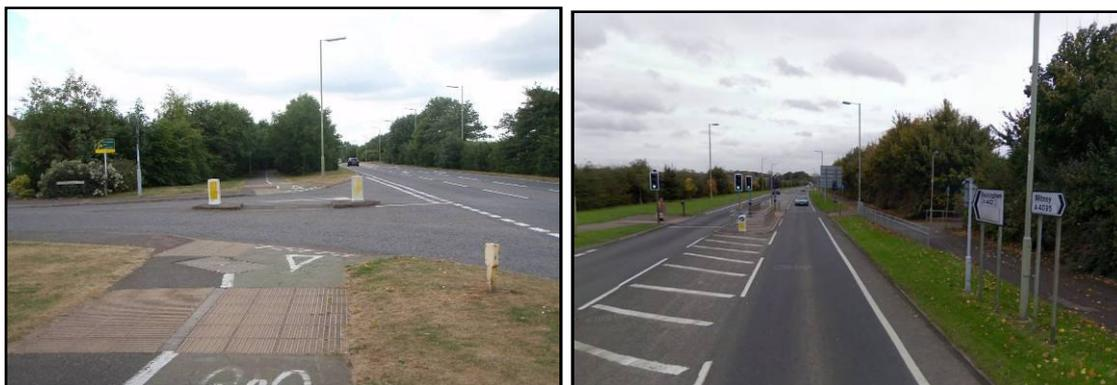
This pedestrian route that aligns the A4095 carriageway is considered to benefit from a good horizontal alignment, street lighting, tactile paving and pedestrian refuges at junctions (as shown in **photograph 3.1**), and is largely clear of vegetation. In addition, the footways that form the route are considered to be of an appropriate width and are well maintained in terms of their
