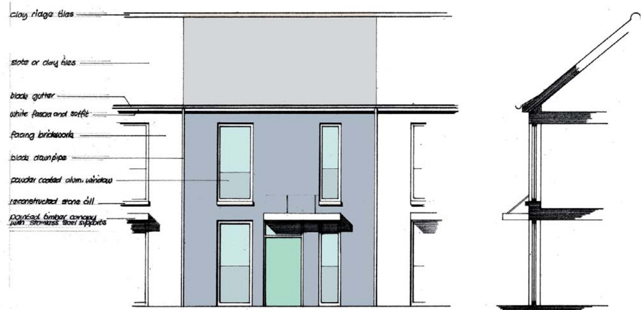
Design Type 2- Part elevation and material labels
