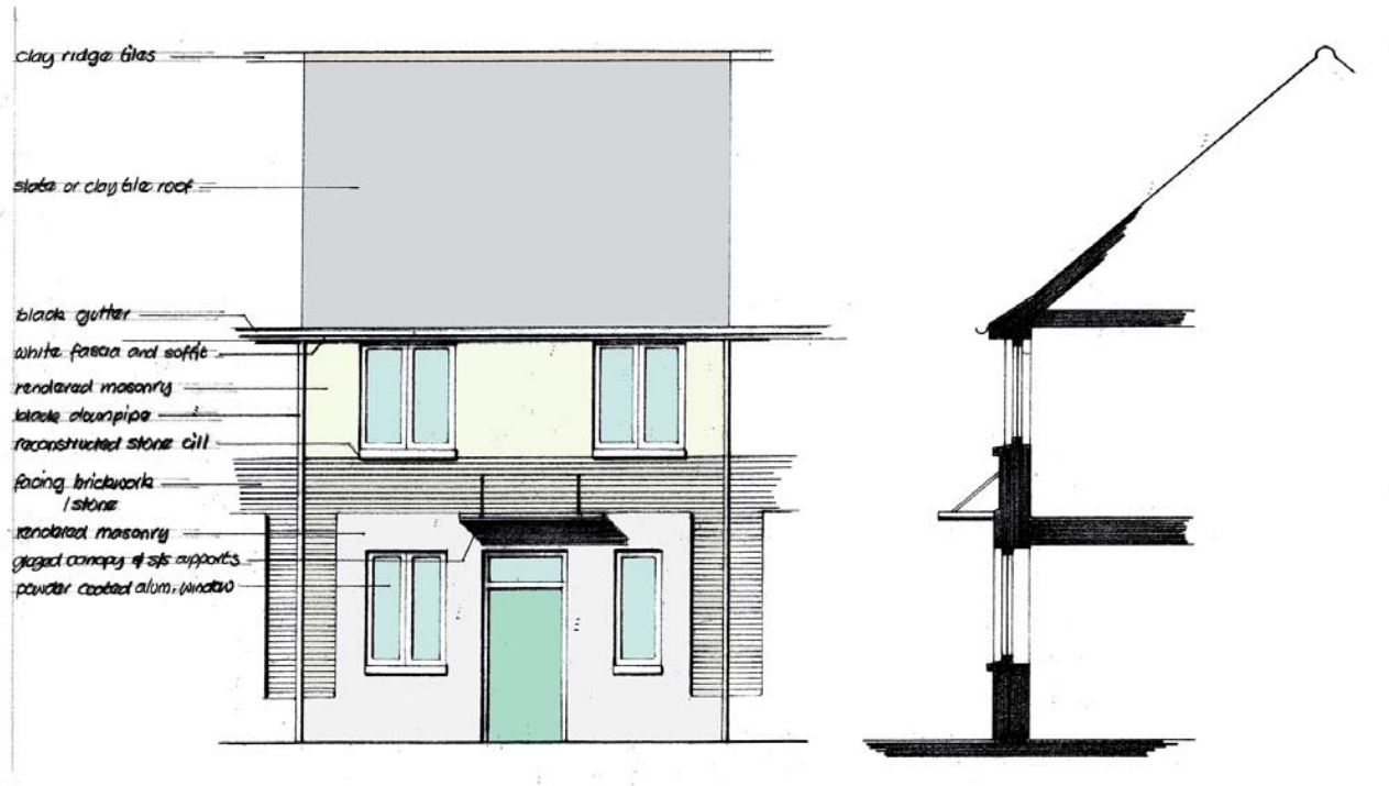
Design Type 1- Part elevation and material labels
