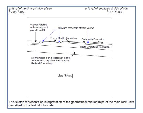
Figure 2-1 Simplified cross section through Exemplar site (BGS 2008)
