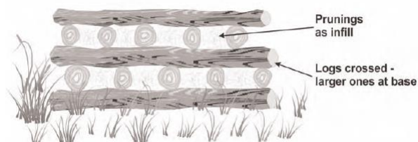
Figure 1.1 Schematic of a wildlife pile (courtesy of Steve Wilson and Robert Bray of Sustainable Drainage Associates)
