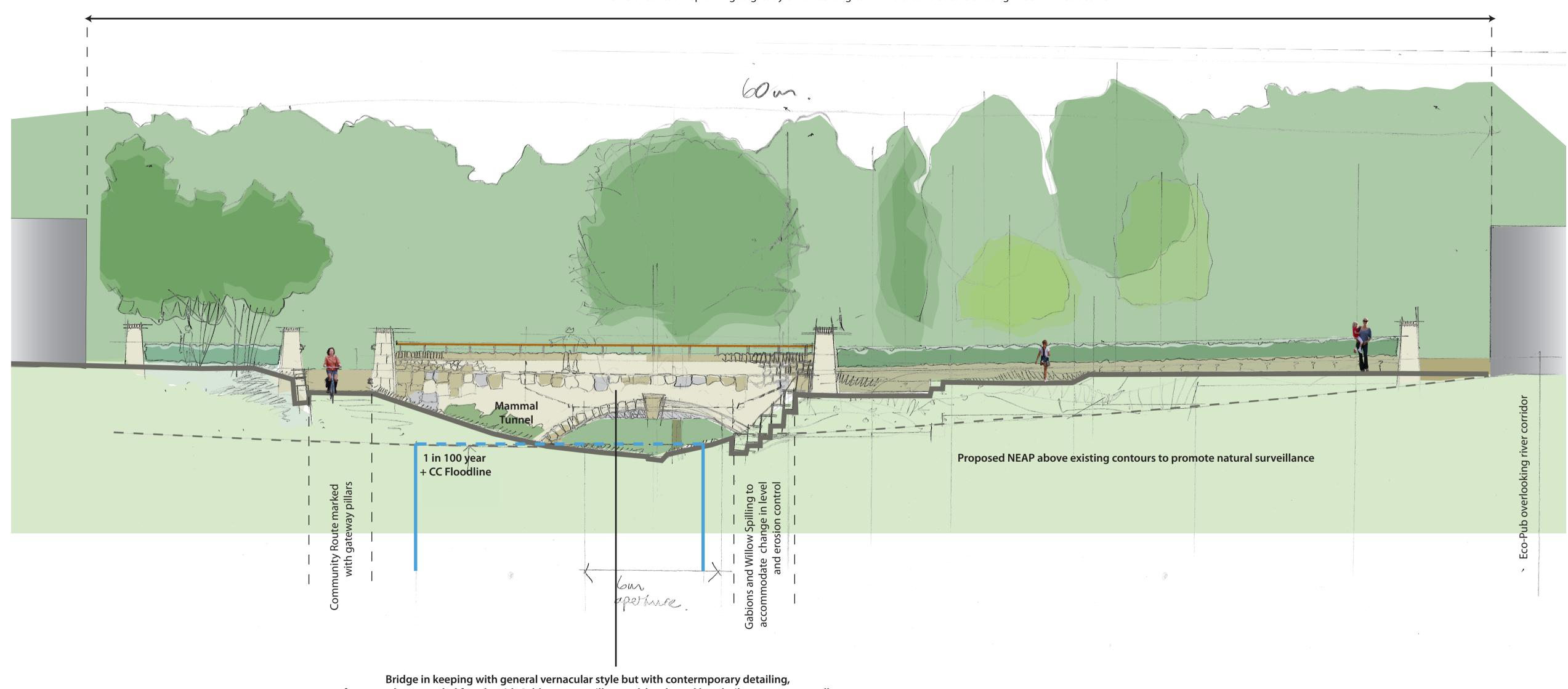
Bridge in keeping with general vernacular style but with contermporary detailing, for example stone-clad facade with Ashlar accent pillars and hardwood handrail atop parapet wall. Stone cladding offers opportunity to incorporate niches and recesses to create micro habitats. Bat-friendly design with under-culvert above watercourse and bat-freindly lighting to parapet wall
