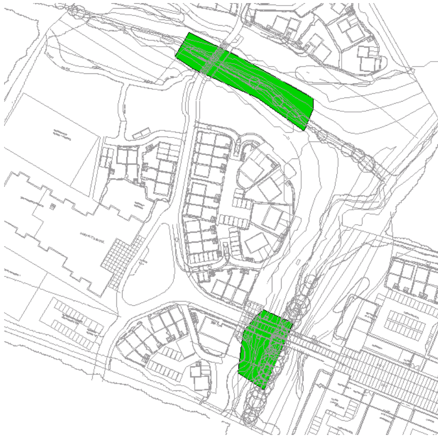
Figure 3-8 Reaches showing increased velocity
