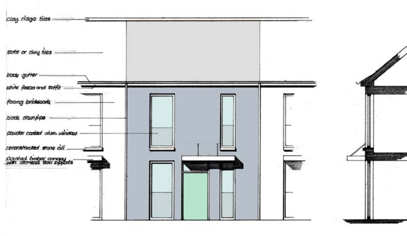
FIG.77 Design Type 2- Part elevation and material labels
