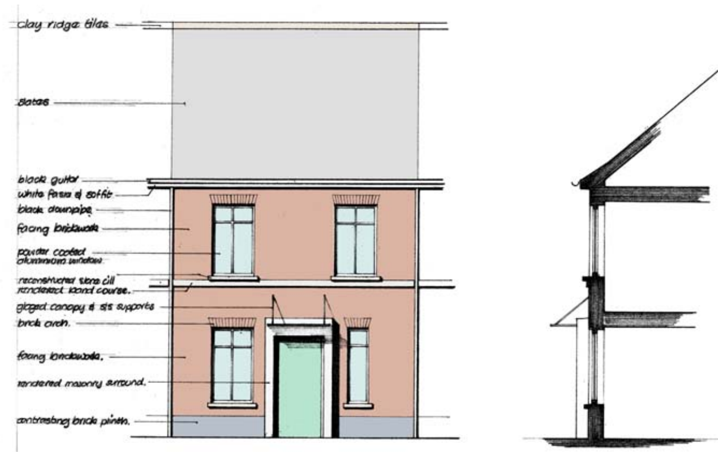
FIG.80 Design Type 3- Part elevation and material labels
