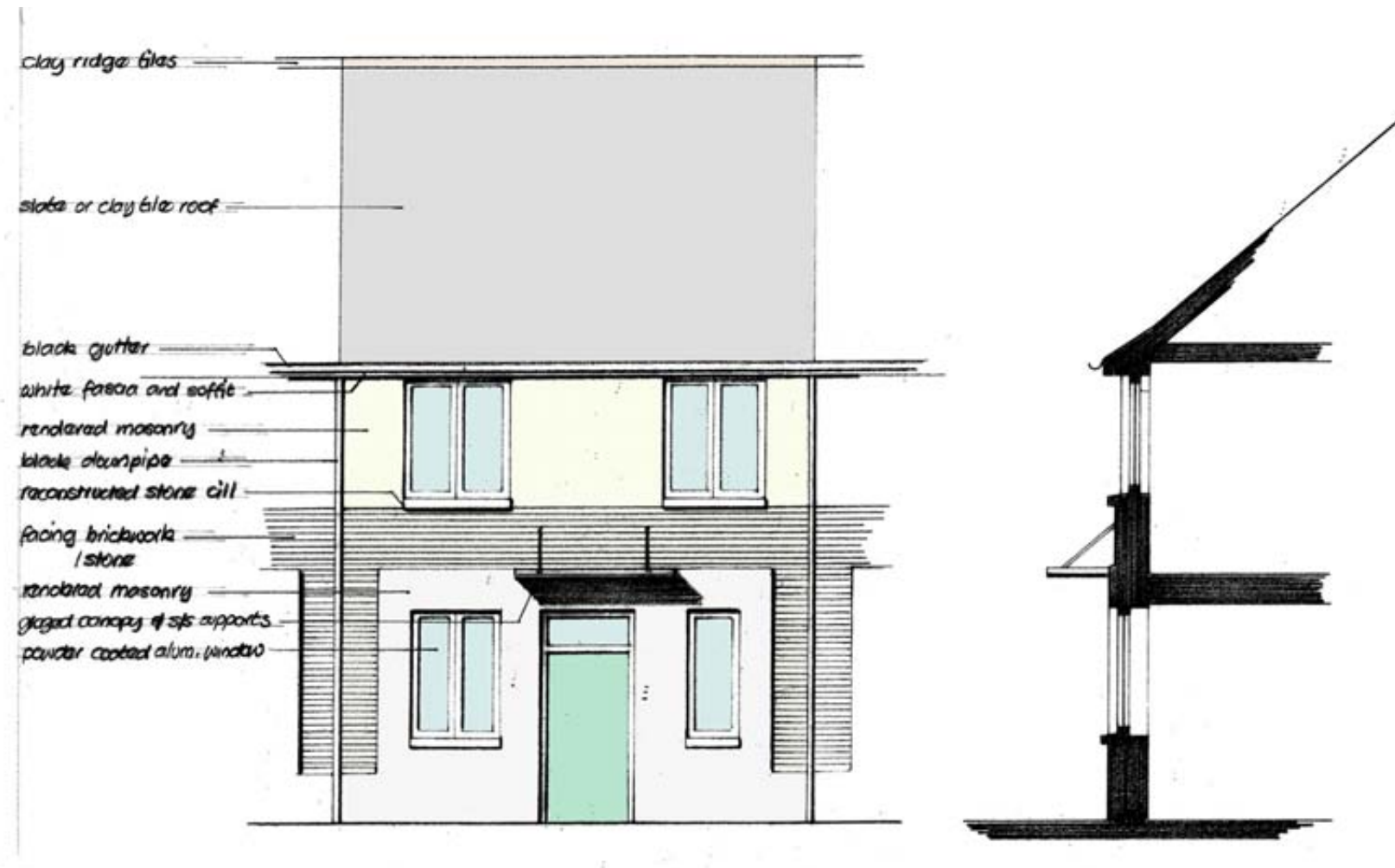
FIG.74 Design Type 1- Part elevation and material labels
