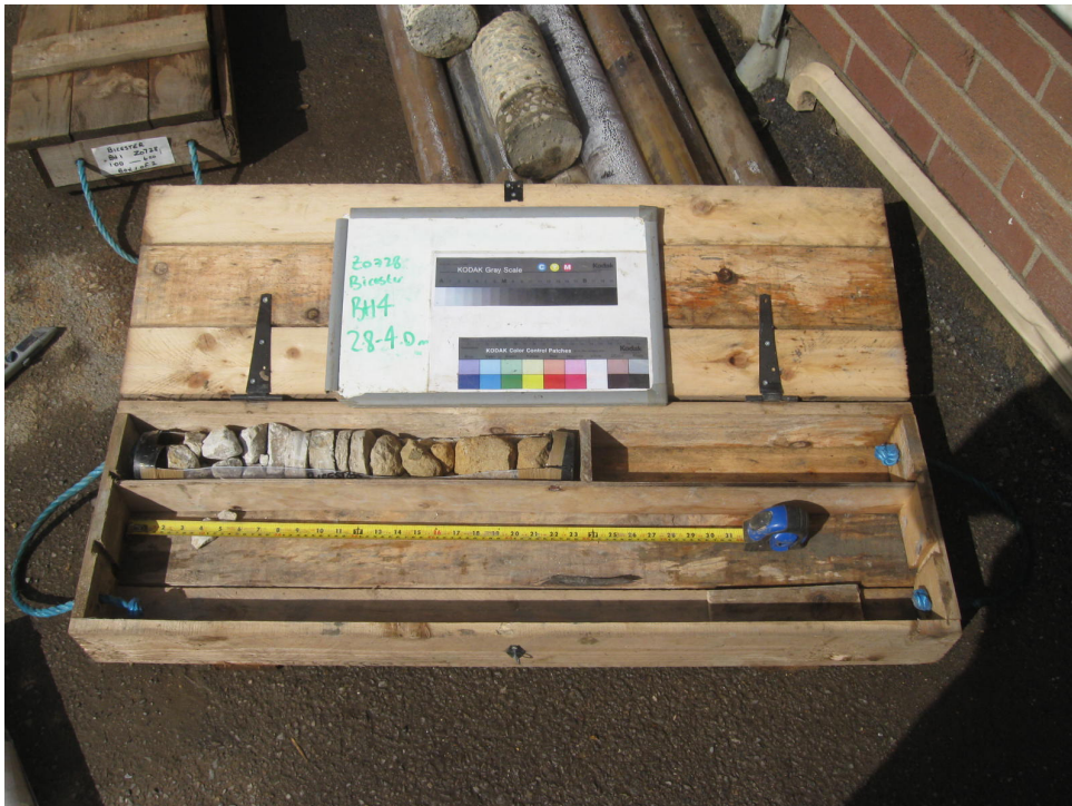
Plate 3: Borehole 4: Box core 2.80m bgl to 4.00m bgl
