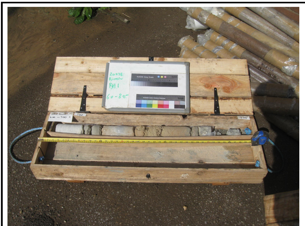
Plate 2: Borehole 1: Box Cores 6.0 m bgl to 8.0m bgl.
