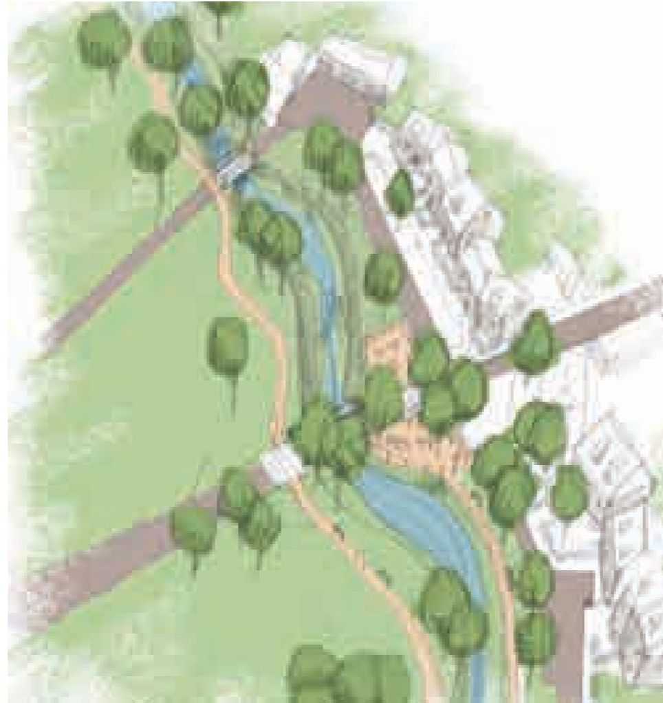
Surface water attenuation will in part be provided by a number of linked ponds. An extensive linear 'nature' park within the western residential area will provide a focus for recreation, play biodiversity as well as providing water attenuation.
