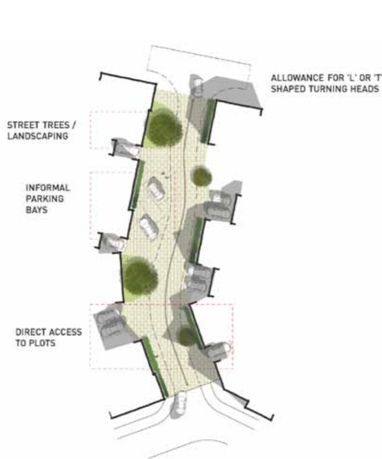
TYPICAL INDICATIVE PLAN SECTION SHARED SURFACE (COMMUNITY STREET) ST.4
