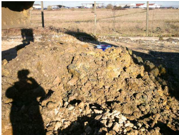
19.01.15 Arising screened with a PID (<0.1 ppm)
