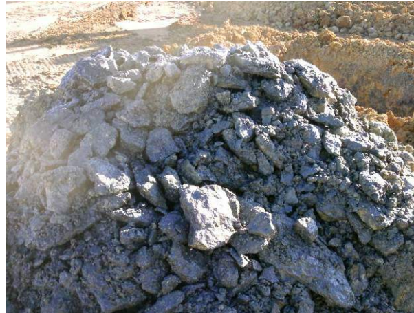
19.01.15 stained gravel encountered with moderate hydrocarbon odour
