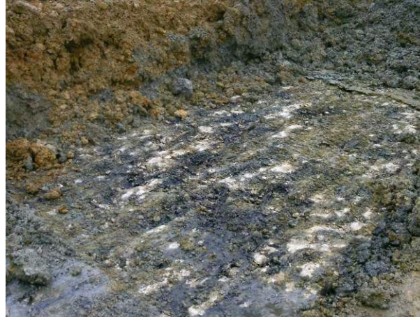
16.02.15 Black staining observed on granular material
