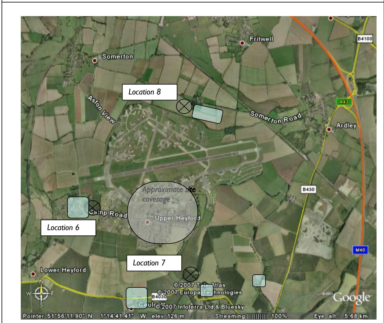
Figure N2: Site plan showing external measurement locations used for setting noise emissions. Blue areas indicate identified residences.
