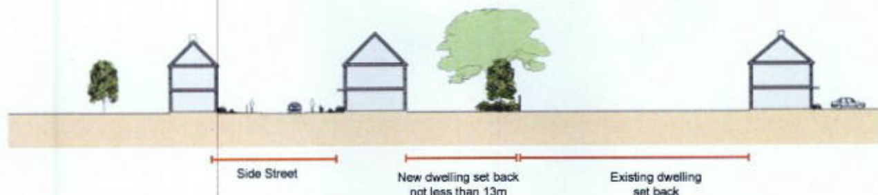
Fig.48: Section 2: Boundary treatment with existing 2 storey dwelling back garden on Oxford Road
