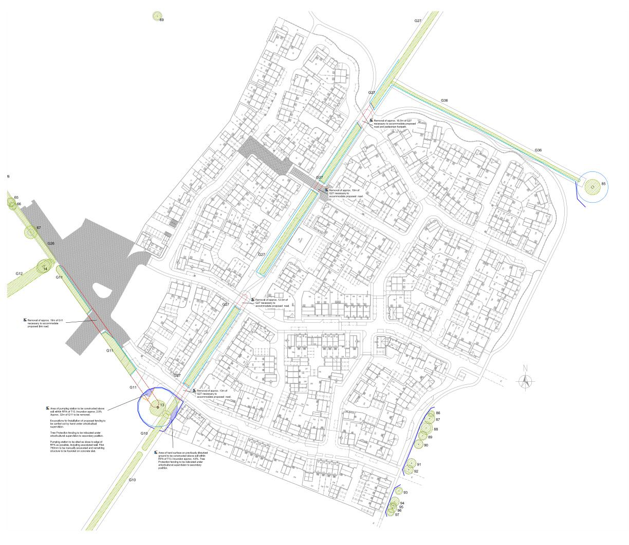
0m 10m 20m KEY: Site Boundary Tree Canopies Category 'B' RPA Category 'C' RPA Trees to be Removed Tree Protection Barrier (Default Specification) Tree Protection Barrier (Secondary Specification) Tree Protection Barrier (2nd Position) Manual Excavation Above Soil Surfacing
