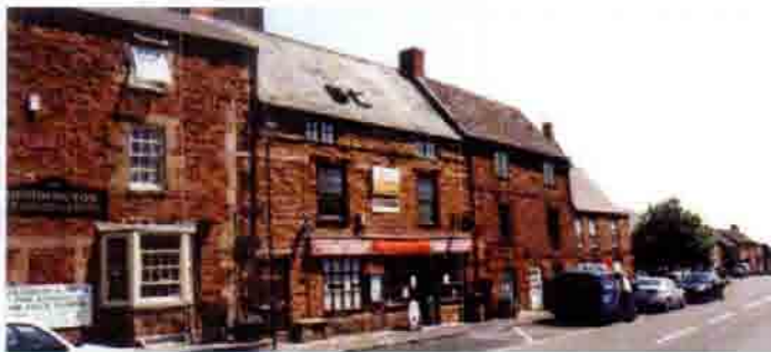
Fig.36: Deddington has a mixed use village centre with a number of shops and services. The ground level shops have slightly larger windows than the residential uses above. Other window features include stone mullions and bay windows. Third storey windows are significantly smaller than at ground level.
