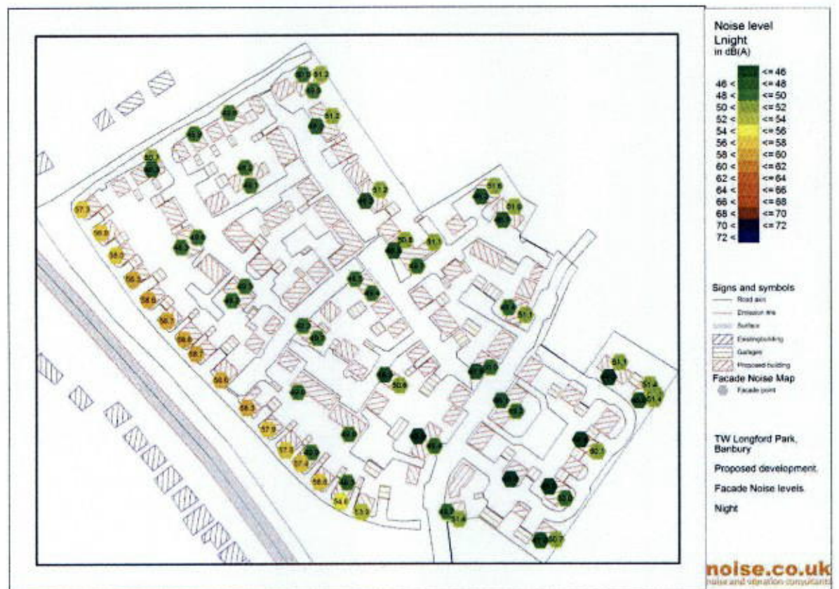
Figure 3 - Facade Levels during the Night-time
