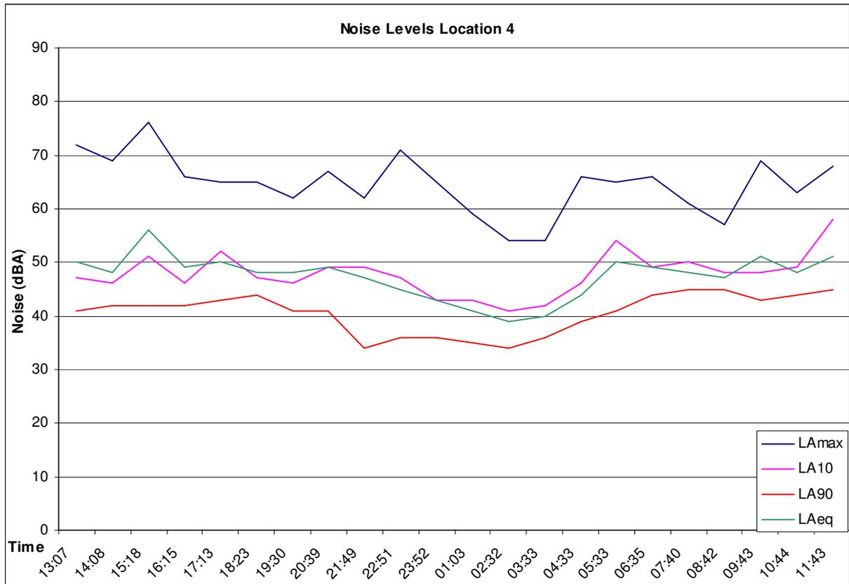
**Figure 6** Graph of L<sub>Amax</sub> L<sub>Aeq</sub> L<sub>A10</sub> and L<sub>A90</sub> noise levels measured at location 4
