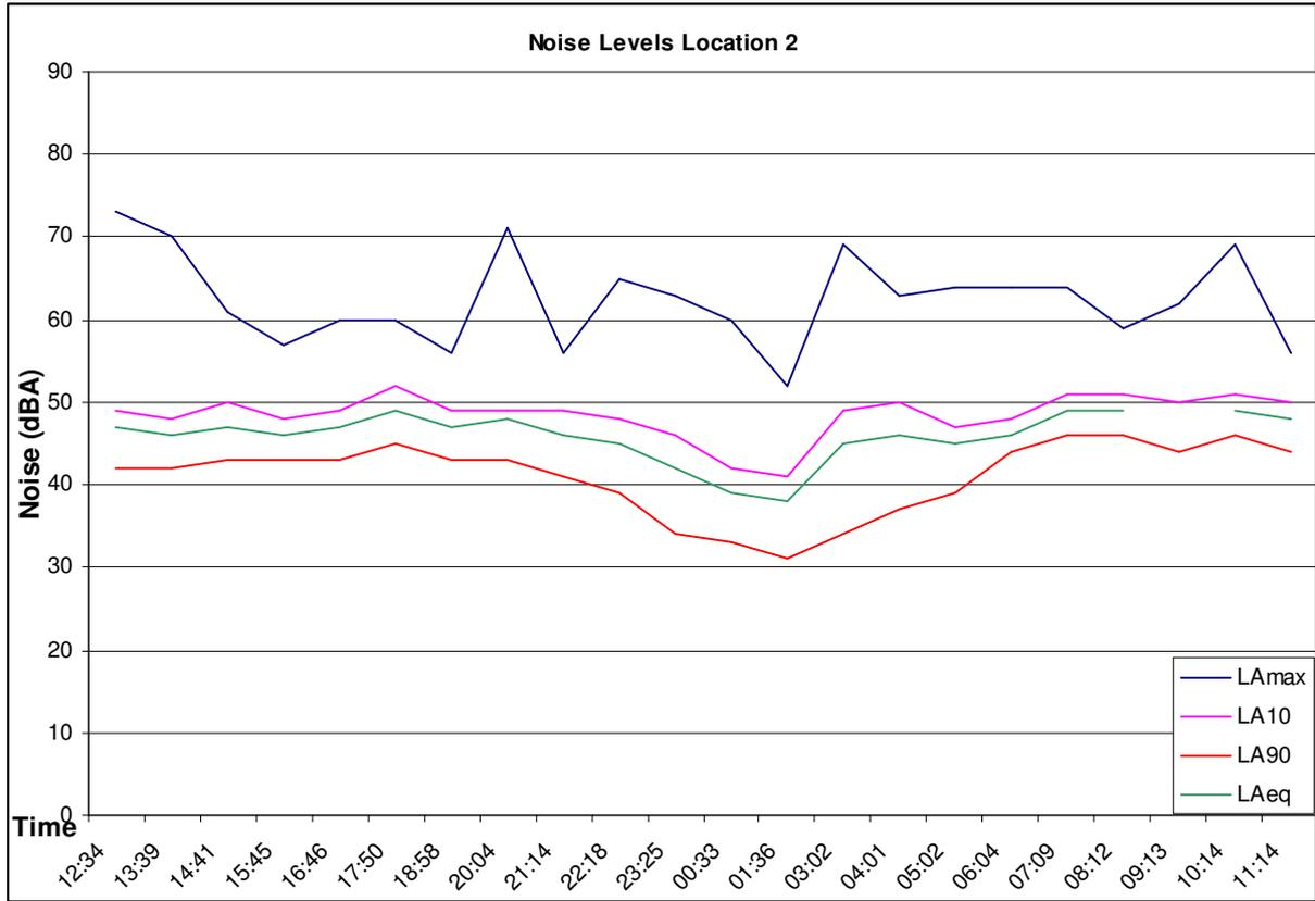
Figure 4 Graph of L<sub>Amax</sub> L<sub>Aeq</sub> L<sub>A10</sub> and L<sub>A90</sub> noise levels measured at location 2
