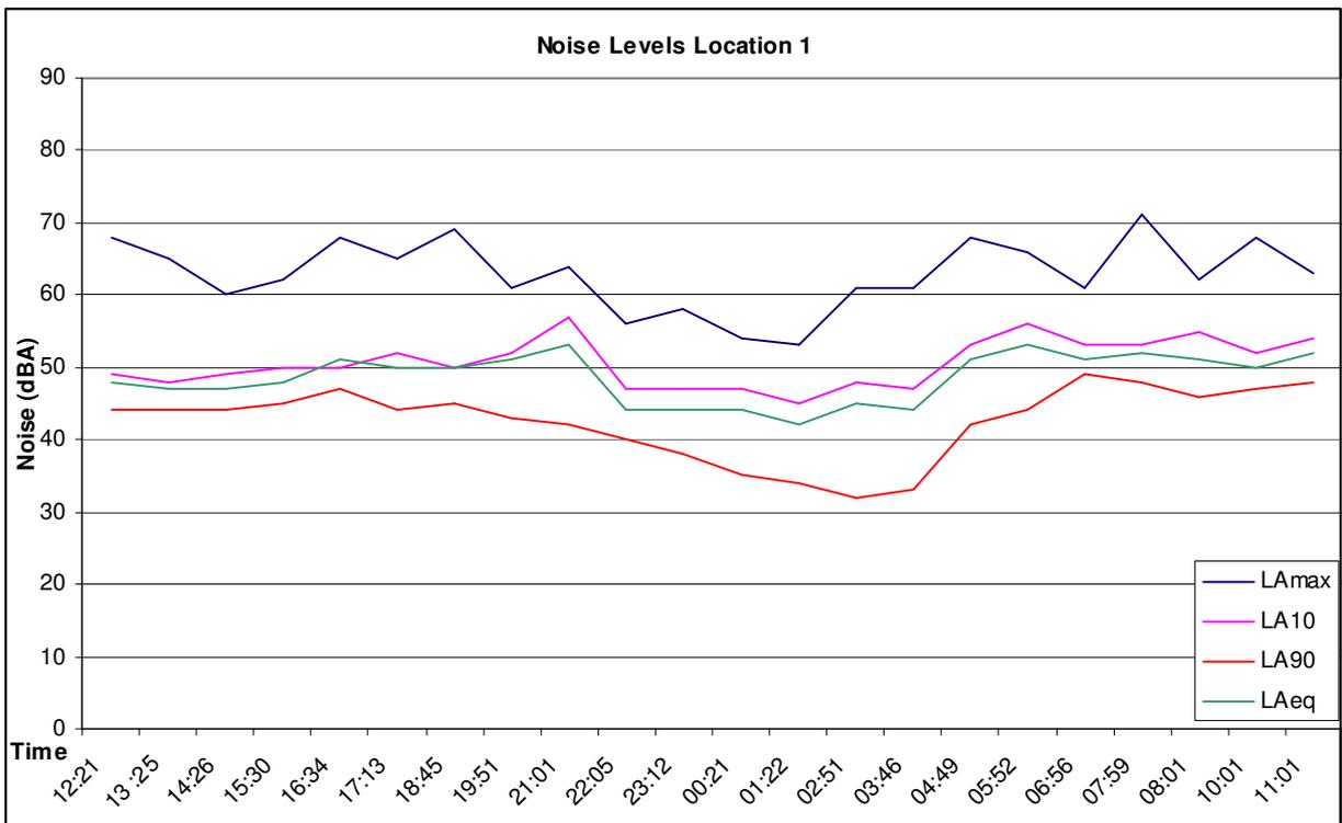
Figure 3 Graph of  $L_{Amax}$ ,  $L_{Aeq}$ ,  $L_{A10}$  and  $L_{A90}$  noise levels measured at location 1
