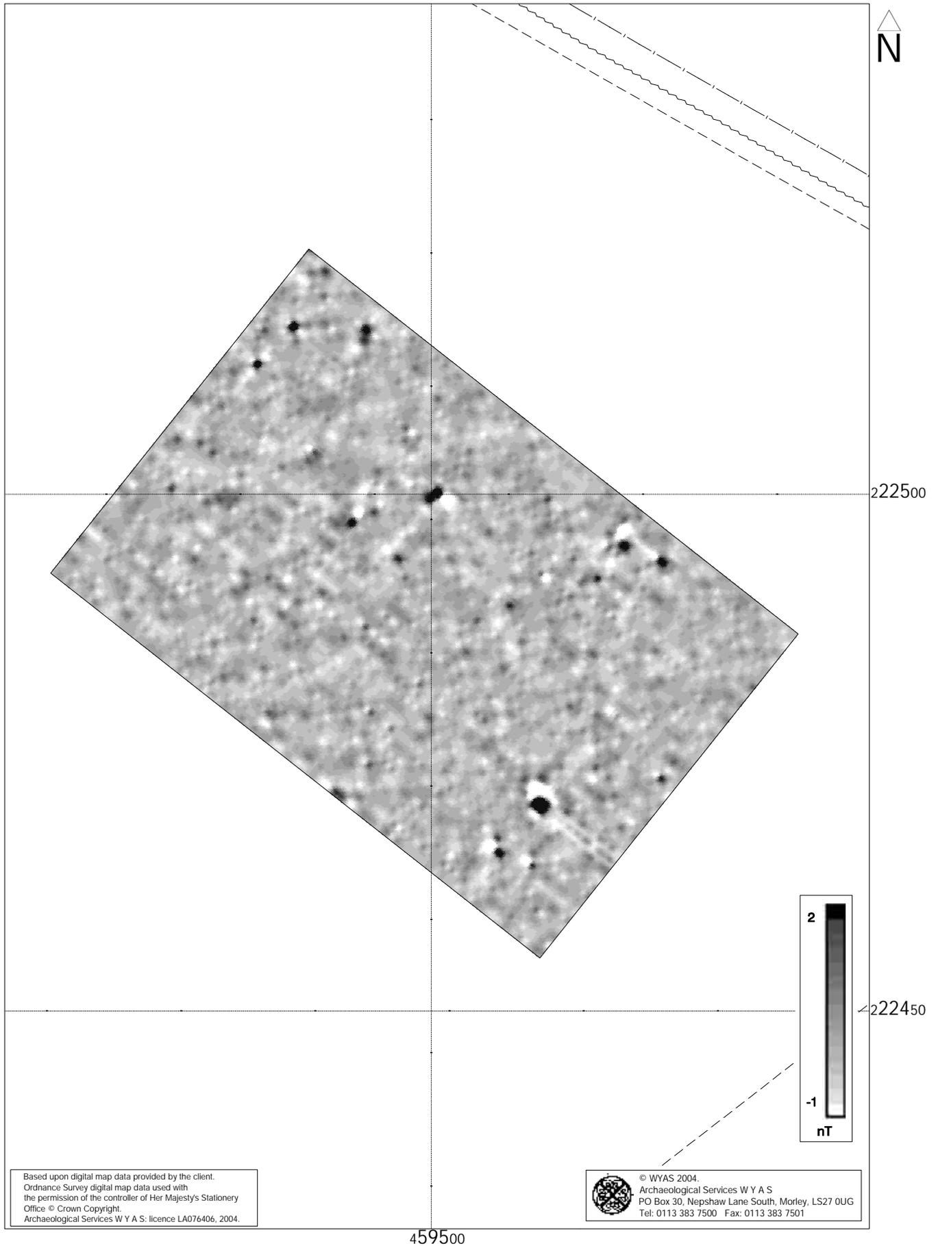
Fig. 3. Greyscale plot of gradiometer data; Block 1
