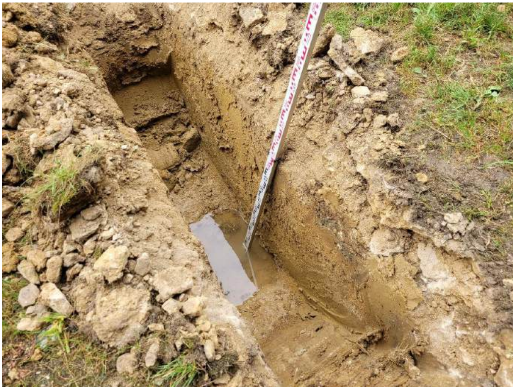
Photo 8 - BRE365 test being undertake in TP3
