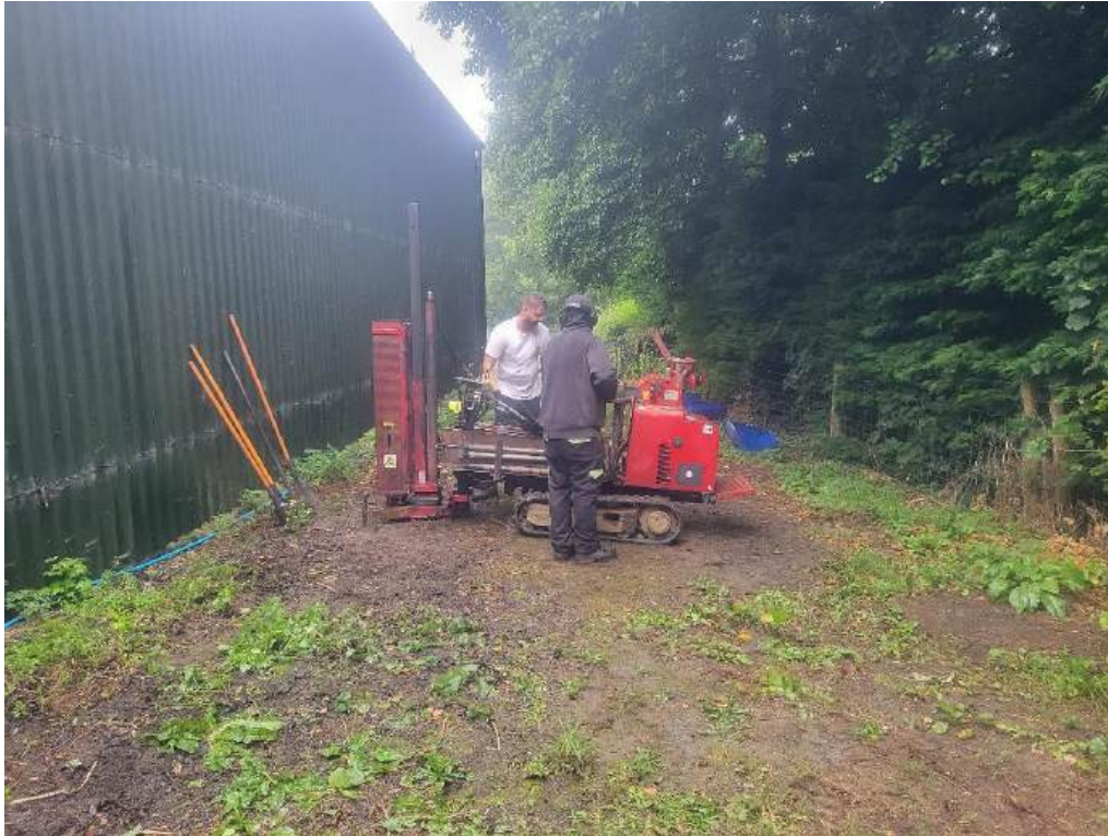
Photo 8 - BRE365 test being undertake in TP3
